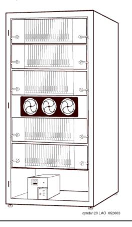
**Single-Carrier Cabinet (SCC1) Media Gateway -** The SCC1 Media Gateway consists of a single carrier. Up to four SCC1 Media Gateways can be connected together in one location to form one port network. There are two types of SCC1 Media Gateways:
